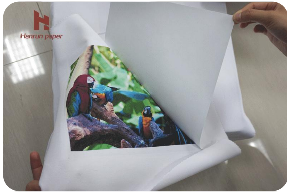
C: Hot peel immediately after transfer
